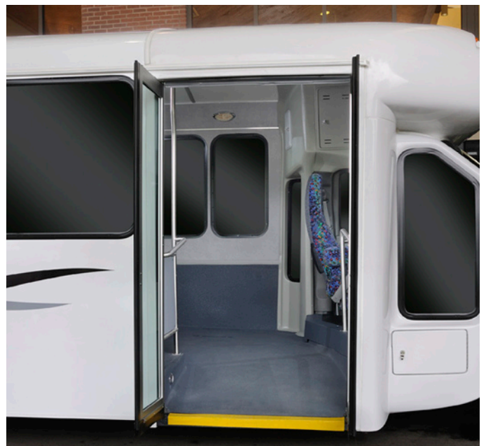
The entrance door width increased to 41 inches on the Spirit LP for easier entrance and exit with luggage.
